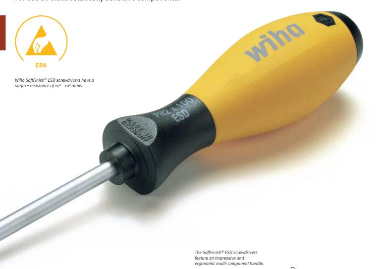
For work on electrostatically sensitive devices and assemblies. there is no better screwdriver than the Wiha SoftFinish® ESD, with integrated soft zone in the multi-component- handle. The dissipative handle with a surface resistance of 106 - 109 ohms discharges the electrostatic energy in a controlled manner to protect devices at risk from electrostatic discharge.
