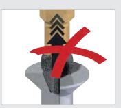
The Dura coatina reduces CamOut effects to an unbeatable minimum no more slipping out of the bit from the screw head.
