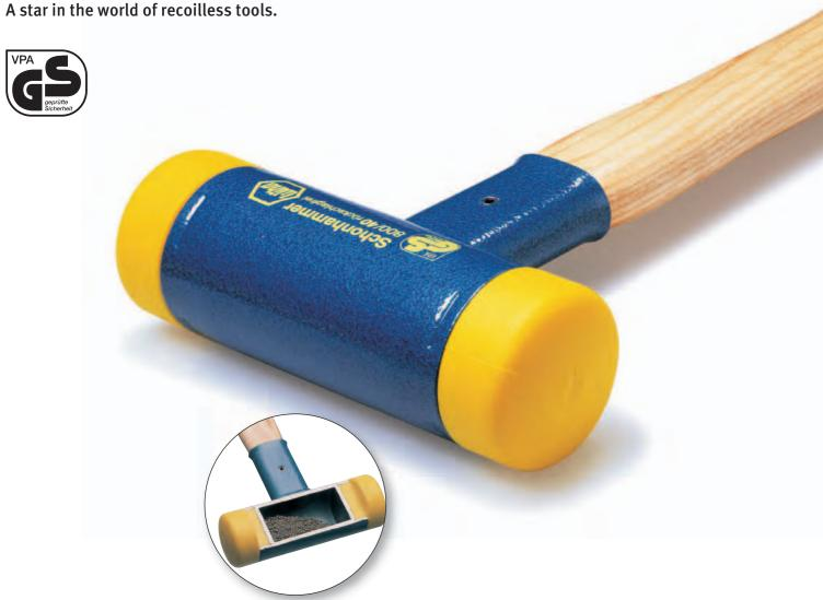
Wiha has now put an end to the familiar problems associated with the stress on joints and muscles when working with recoiling hammers. The Wiha dead-blow hammer has a special filling in the hammer casing to prevent recoil. Professionals who use these hammers on a continuous basis, for example, in tool and die shops or in body maintenance and sheet-metal work, appreciate the benefits of this recoilless hammer from Wiha.
