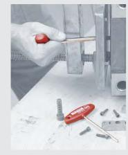
A wide range of hex (metric and inch sizes), TORX® and TORX PLUS® blades, as well as hex drivers (metric and inch), ensures that the perfect tool is at hand for all conceivable applications. A colour-coding system for the handles facilitates the selection of the right blade.
