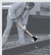
The powder-coated safety shells made from malleable cast iron clamp the head and handle securely together. The 840 mm long sledge hammer is the ideal length for special applications,
