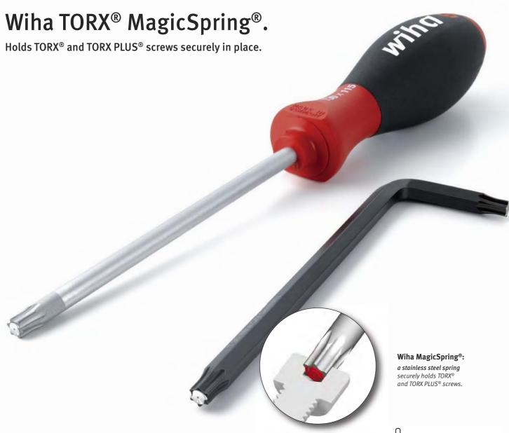
No more annoying and timeconsuming hunting around for TORX® or TORX PLUS® screws that have apparently vanished into thin air. With Wiha's ingenious new tool, the MagicSpring®, TORX® or TORX PLUS® screws\* are kept firmly where you want them. The highlight of the "MagicSpring®" tools is the stainless steel "magical" retaining spring that, together with a thin cover disc, is laser-welded to the tip of the blade.
