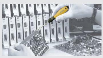
The hard handle core consists of impact resistant polypropylene. The thermoplastic elastomer handle provides for a pleasant, safe and slip-proof grip. The inseparable handle is connected to the core by a moulding process. The high-quality blade of chromevanadium- molybdenum steel is through hardened and mattechrome plated. The Wiha ChromTop® blade tip ensures a perfect fit in every screw head.
