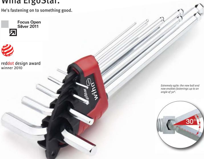
The trick with the new Wiha ErgoStar is as simple as it is effective: rotating a single L-key in the holder means that all other keys rotate to the side at the same angle! That means: there's no more complicated disentangling of adjacent keys any more. All L-keys are ready for removal with a single turn, quicker, more simply and more clearly than ever before.
